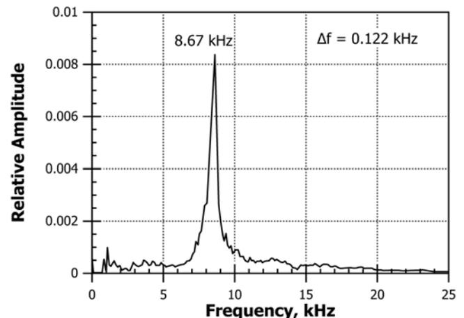
FIG. 5 Waveform and Amplitude Spectrum for Valid Impact-Echo Test of 250-mm Thick Concrete Slab
