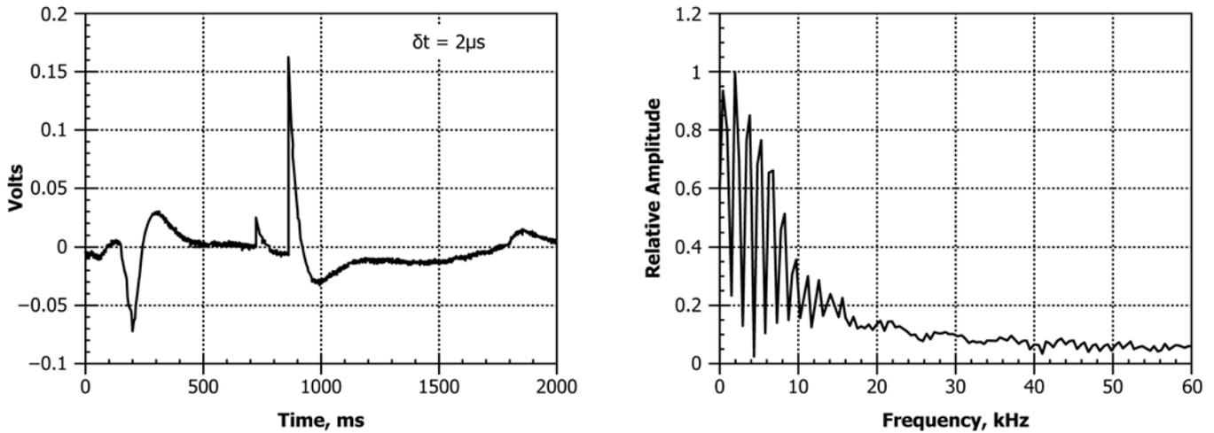
FIG. 6 Example of Invalid Impact-Echo Test, Waveform Does Not Display Periodic Oscillations and Amplitude Spectrum Does Not Have Single Dominant Peak
